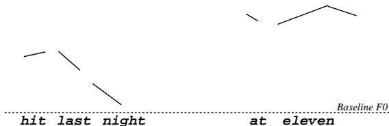
Fig. 4: Schematic example of stylized F0 for voiced regions of the text. The speaker’s estimated baseline F0 (from the lognormal tied mixture modeling) is also indicated.
